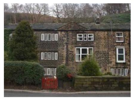
Laneside House, Rochdale Road - The Fieldens' first spinning mill. Note the blocked up 'taking in' door in the centre of the upper floor.
